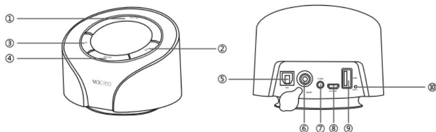
1. Mode Button: Press to switch between working modes, or press and hold for 5 seconds to switch between 3.5mm analog line-out or OPT&SPDIF digital output.
